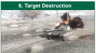
The XM204 TA autonomously engages vehicles through ground based and submunition sensors. Once manually armed, the XM204 TA system autonomously detects, tracks, and can engage multiple target vehicles using seismic, acoustic, radar sensors, and a top attack explosively formed warhead.
